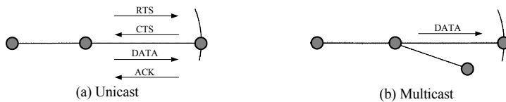
Fig.1 Comparison of packet exchanges at MAC layer during unicast and multicast routing
