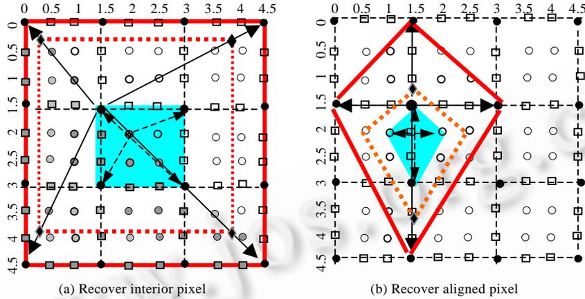
Fig.3 Determination of the neighboring window and the training window (magnification factors of 1.5)
