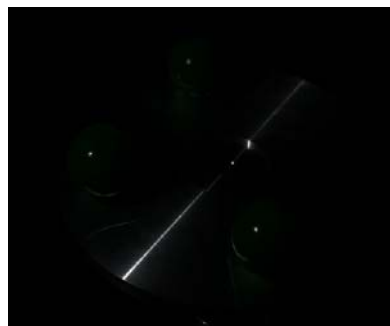
(b) Exposure time 1/200s, used to calculate the light source position via the specular spike points
