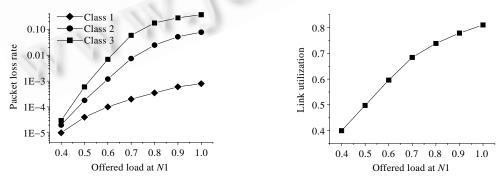
Fig.6 Packet loss rate for three classes at node *N*1
