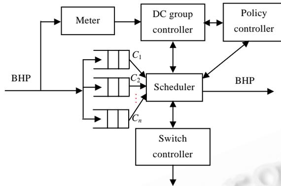
Fig.1 Functional model of the core node
