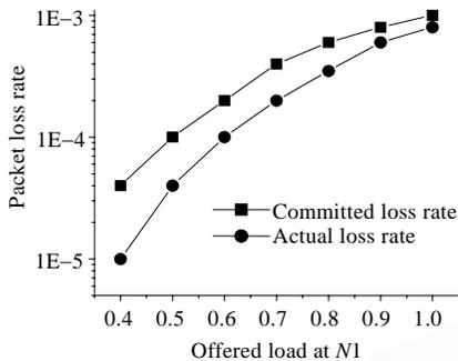
Fig.8 Committed packet loss rate and actual packet loss rate for class 1
