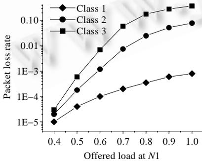
Fig.6 Packet loss rate for three classes at node  $N1$
