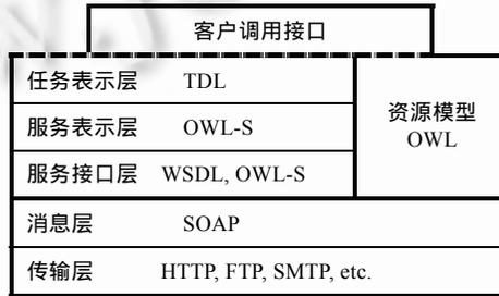
Fig.1 Task goal-oriented service representation model protocol stack
