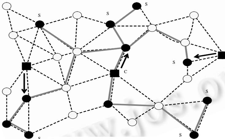
Fig.8 Multicast tree is composed by all servers and thick lightly shaded lines
