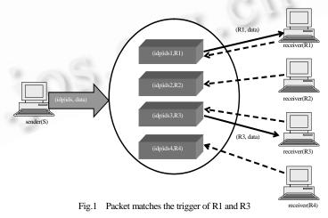
(using IP) between I3 nodes and to end-system. Identifiers and triggers have meaning only in this overlay network. Figure 1 illustrates manycast in I3 (Reproduction based on Fig.2c in Ref.[28]). The dashed directional lines represent triggers and solid directional lines indicate the data transmissions.
