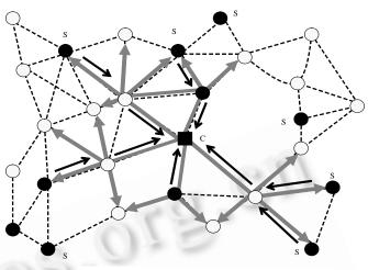
Fig.3 Scoped-flooding with TTL=2 can find 7servers
