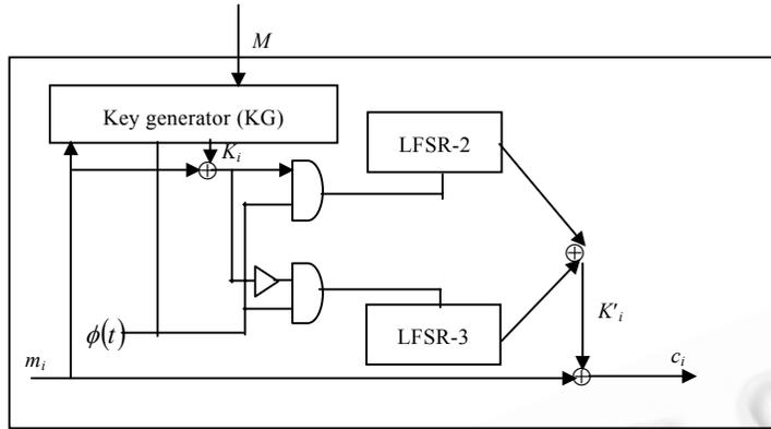
Fig.4 The stream cipher S3
