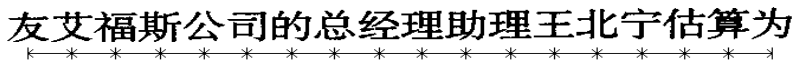
Fig.2 The equidistance between centers of Chinese characters 图 2 汉字字符中心的等间距性
