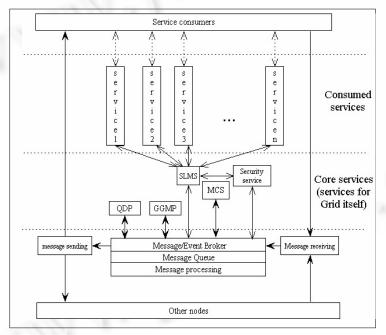
Fig.5 Message-Based implementation of VDHA\_Grid
