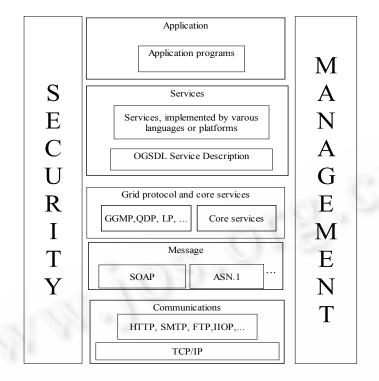
Fig.3 VDHA Grid architecture
