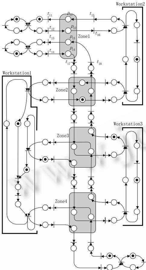
Fig.4 The automated guided vehicle PN
