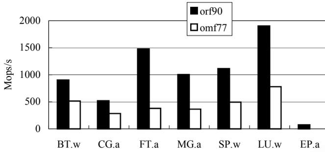
Fig.6 Performance comparison on NPB3.0 OpenMP FORTRAN suite. Mops/s means Mega-operations per second, the metric defined by NPB, and the higher, the better. orf90 is our OpenMP compiler based on ORC2.0<sup>[11]</sup>, and omf77 is Omni OpenMP compiler(1.4a). The individual benchmark name is in a form like BT.w. BT is the application name, and w stands for a problem size. Both with `-O3` enabled
