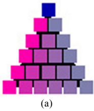
Fig.6 Rasterized points without antialiasing
