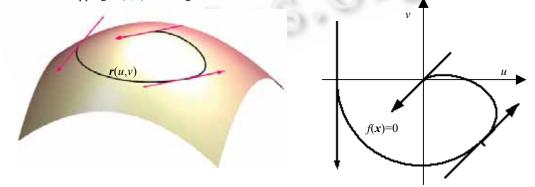
Fig.7  $G^2$  continuous interpolation curve on a paraboloid Fig.8 The original image curve on parametric plane
