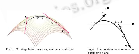
Still taking a paraboloid as an example, we construct a surface interpolation curve passing the given end points with the specified tangent directions and curvature vector at the end points.
