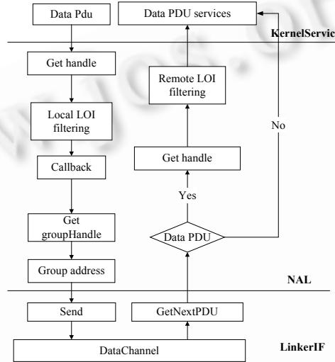
Fig.3 Filtering logic based on the LOI in NAL
