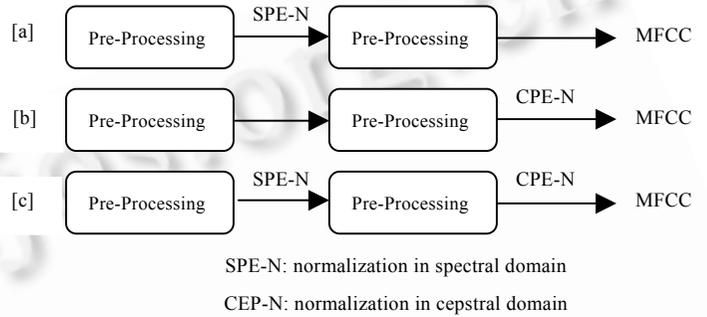
Fig.1 Normalizations in spectral and cepstral domains
