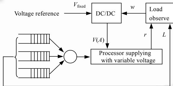
Fig.4 DVS power control principle
