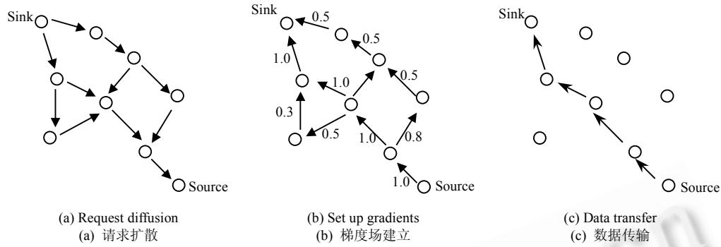
Fig.3 Principle of directed diffusion routing
