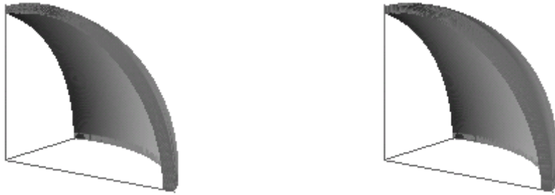
(a) Original one eighth approximate interval spherical surface (of order 5) (a) 原始 1/8 拟区间球面(5 次) (b) Interval triangular Bézier surface after degree reduction (of order 4) (b) 降阶后得到的区间三角 Bézier 曲面(4 次)
