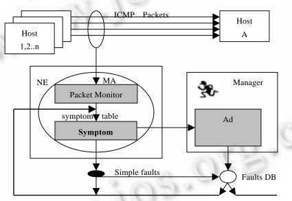
Fig.3 The structure of the intelligent mobile agent
