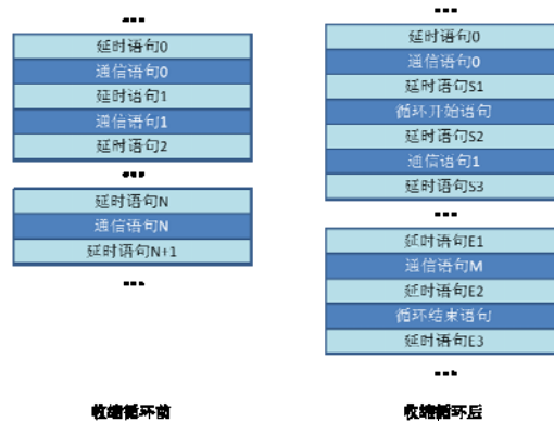
Fig.2 Adding delay statements after repeat-compression
