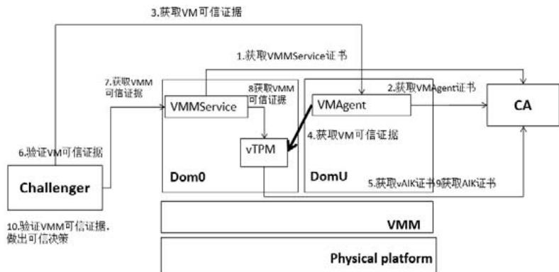
Fig.15 Architecture of experiment of trusted virtual platform remote attestation
