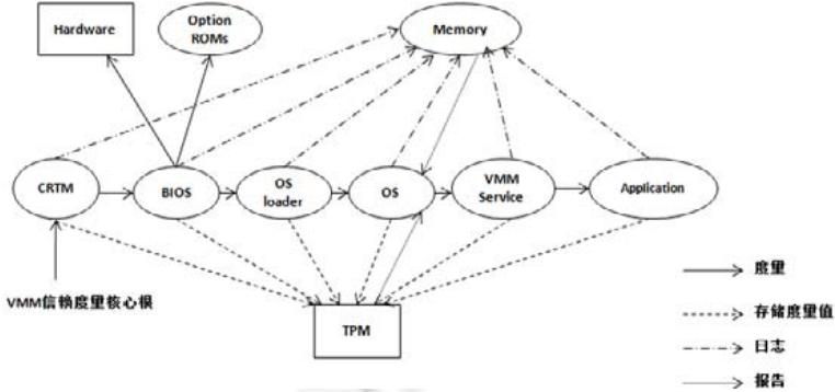
Fig.8 Measurement of attestation service by TPM
