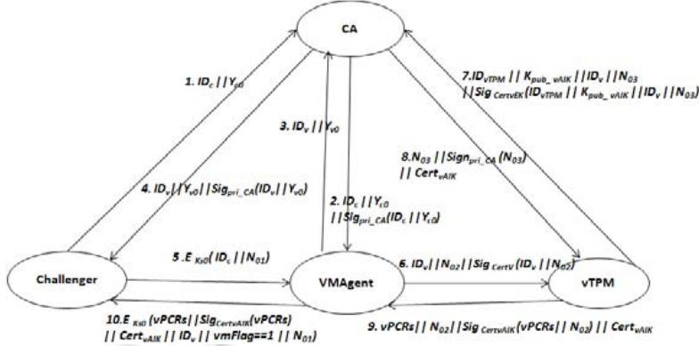
Fig.4 Process of virtual machine remote attestation
