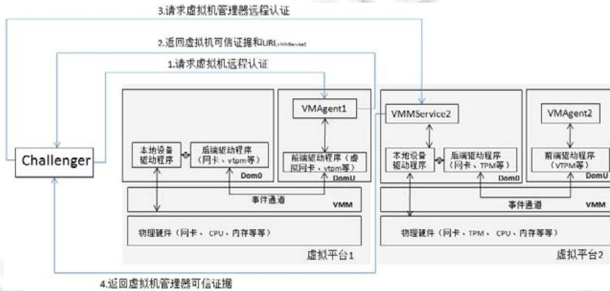
Fig.10 Process of the untrusted virtual platform remote attestation (1)
