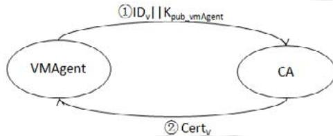
Fig.2 Initialization of virtual machine remote attestation agent
