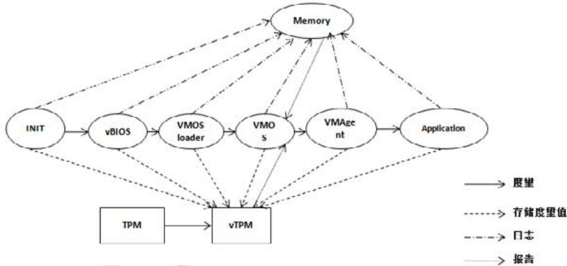
Fig.6 Measurement of attestation agent by vTPM
