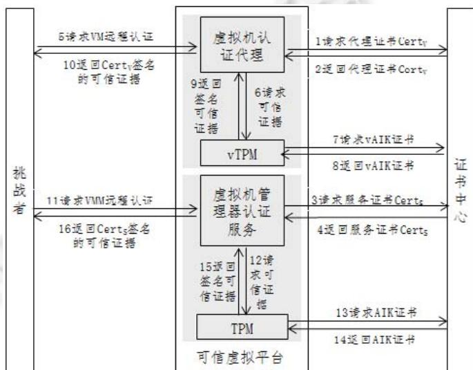
Fig.1 Trusted virtual platform remote attestation method
