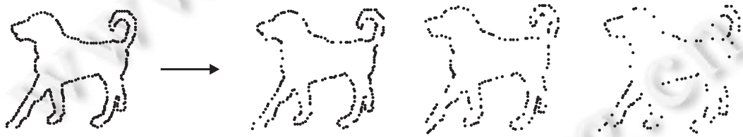
Fig.6 Three contours (from the second left Figure to the fourth left Figure) obtained by randomly removing 20%, 40% and 60% of the points of the original dog shape contour (the first left Figure), respectively
