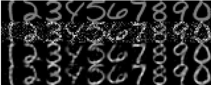
Fig.3 De-Nosing results obtained by different methods (1st row: original image; 2nd row: noisy image; 3rd row: de-noising result by batch KPCA; 4th row: de-noising result by proposed method)
