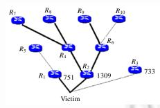
Fig.5 Attack tree, thick lines are parts of the attack paths while thin ones are not
