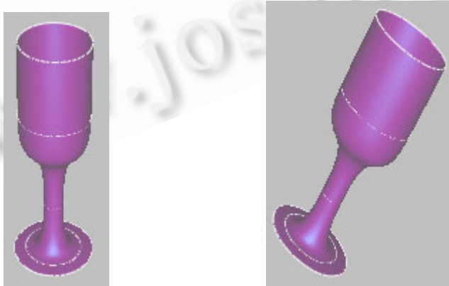
Fig.14 The goblet. Subdivision surface interpolating multi nonintersecting curves, where the highlight curves are the interpolated curves
