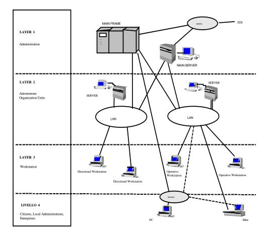
Fig.8 Logical architecture of the FIS information system
