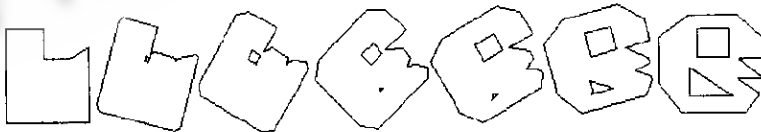
Fig. 5 Generalized morph-interpolation result of two polygons. The middle 5 polygons are the results of generalized morph-interpolation, while r=5/6, 4/6, 3/6, 2/6, 1/6 , respectively.
