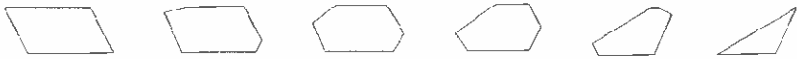
Fig. 1 The metamorphosis of two convex polygons, the middle 4 polygons are the results of rA \oplus (1-r)B while r = 4/5, 3/5, 2/5, 1/5 respectively
