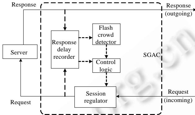
Fig.4 Architecture of SGAC
