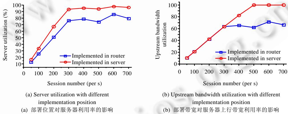
Fig.16 Impact of implementation position to the server and upstream bandwidth utilization
